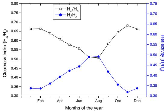
**Fig. 6. Comparison between the reflectivity ( $H_r/H_0$ ) and the clearness index ( $H_m/H_0$ )**
