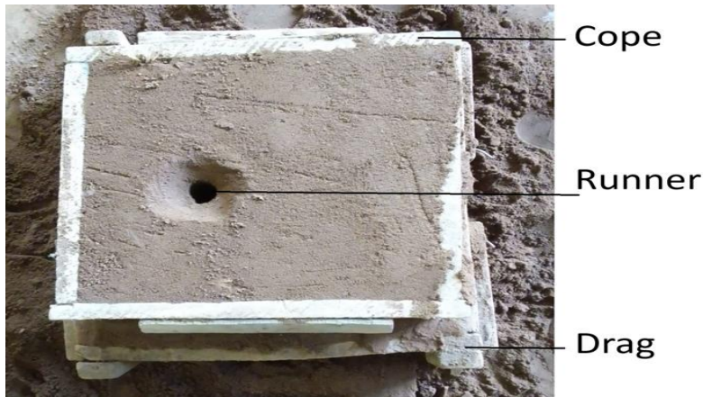
Plate 1. Assembly of Cope and Drag Showing the Runner
