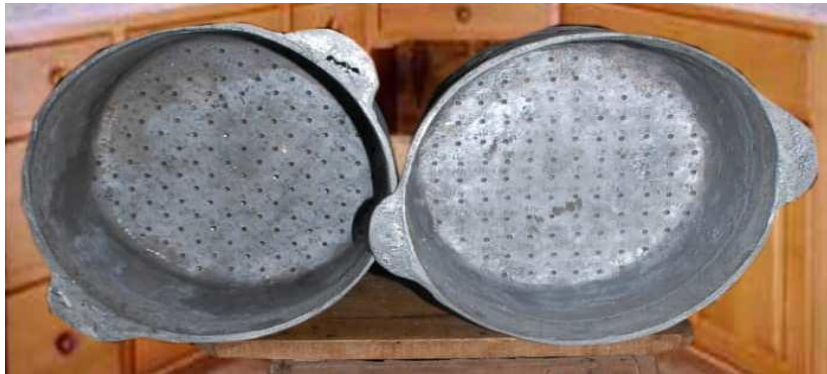
Plate 4. 7-litre EABPs Showing the Internal Cylindrical Fins' Potential Placement Locations
