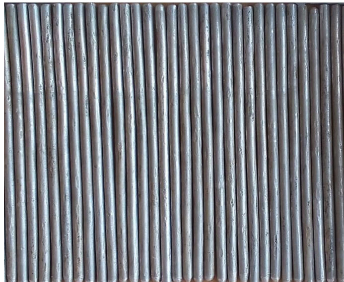
Plate 5. Heat Transfer Internal Cylindrical Fins (Ø5 × 140 mm)
