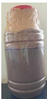
Fig. 1h. Anaerobic fermentation of FW slurry for 14 days
