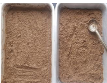
Fig. 1j. Mixing of DORB (Slurry: DORB, 7:1)
