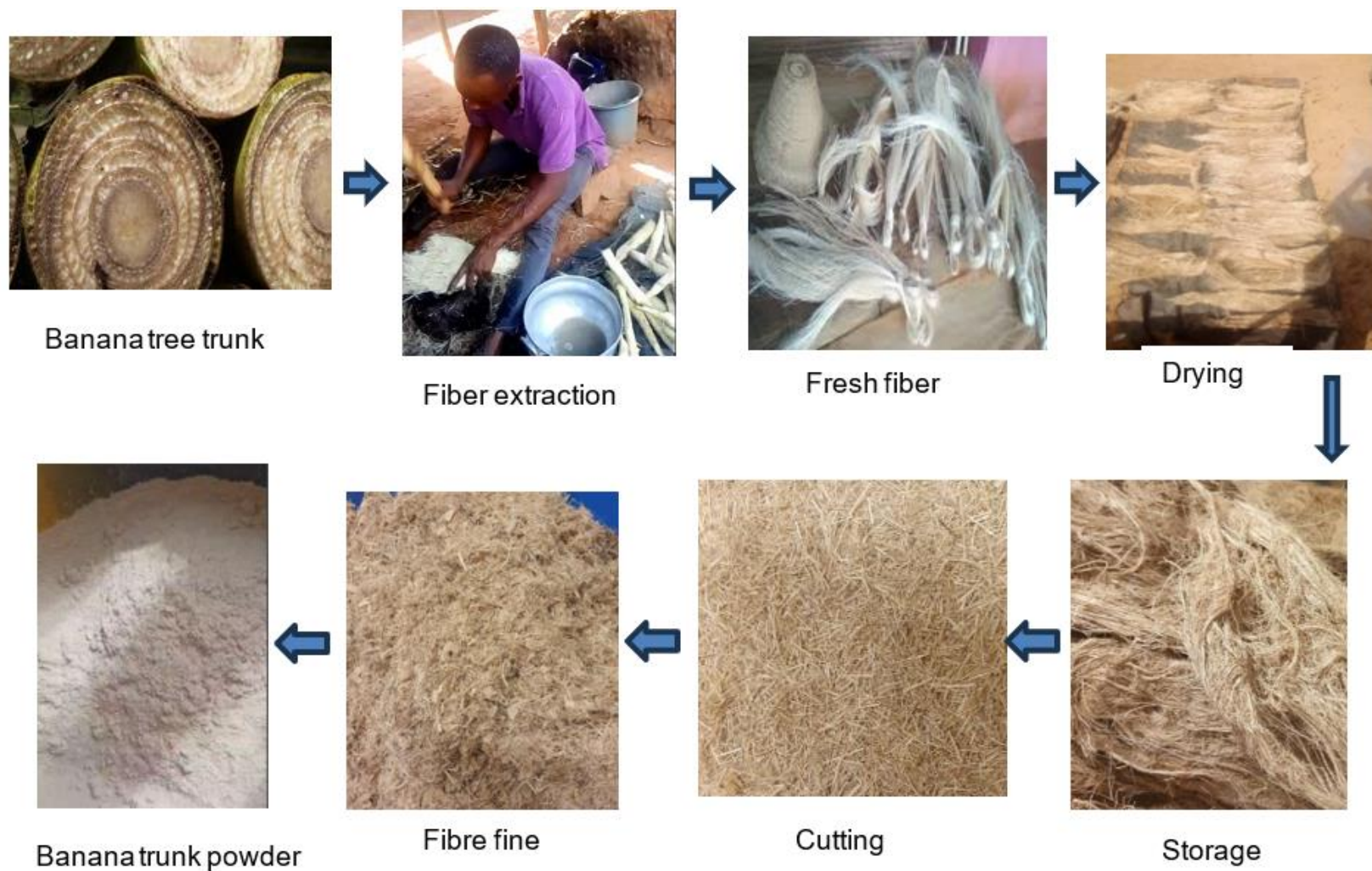
Fig. 4. Banana trunk powder production flow chart
